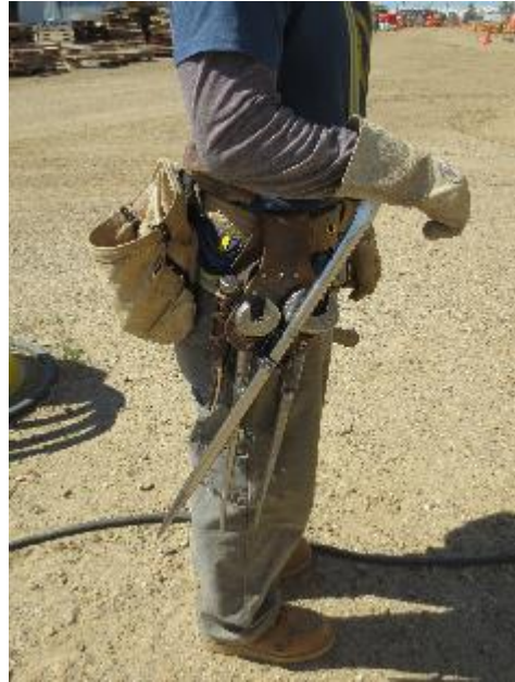
Figure 2: The Industrial 1st Year Apprentice Ironworker's typical tool belt.
