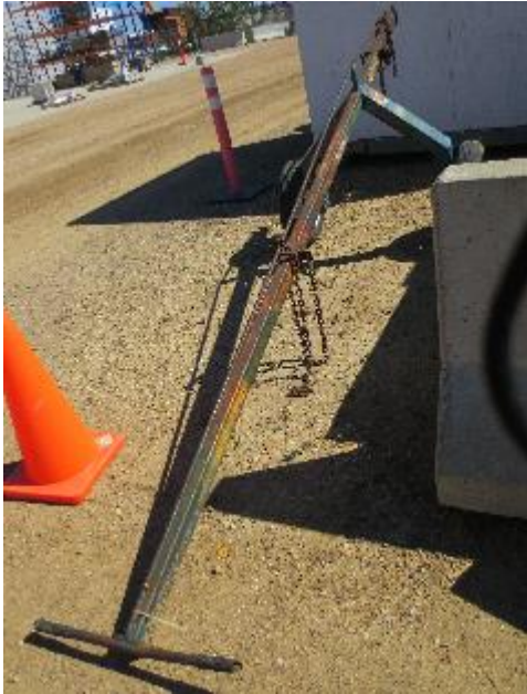
Figure 3: Sorting hook attached to cable used to rig the bent and allow the crane to pick up the structural steel.
