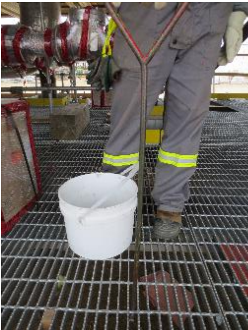
Figure 7: Grating hook used to move the grating onto the open hole. Typically used with a second person; one on each end of the grating.
